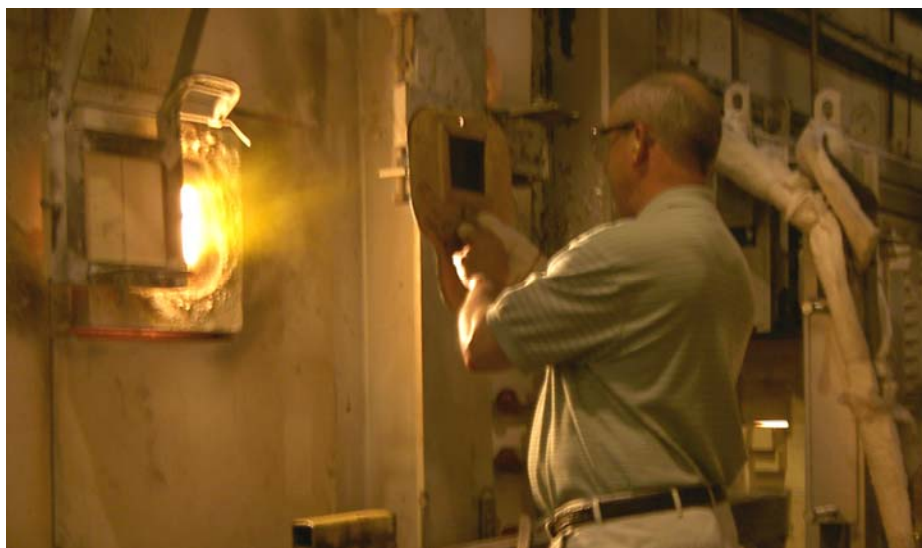
Steve Burgess of Brin peers into the melter to see molten glass at the beginning of the float process - Cardinal Float Plant tour . (See more on page 4)
